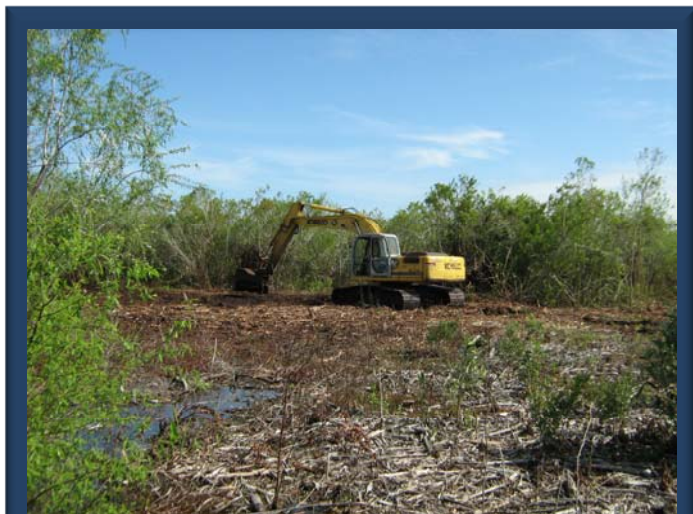
Brontosaurus treatment of shoebutton Ardisia in Miami-Dade County. Photo: Miami-Dade County EEL Program.
