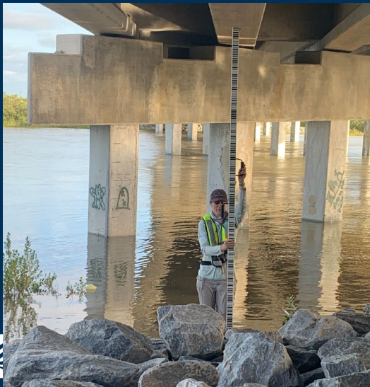
USGS hydrologic technician Megan Bock surveys high water marks from Hurricane Ian in Marineland, Florida. Photograph taken October 4, 2022.
