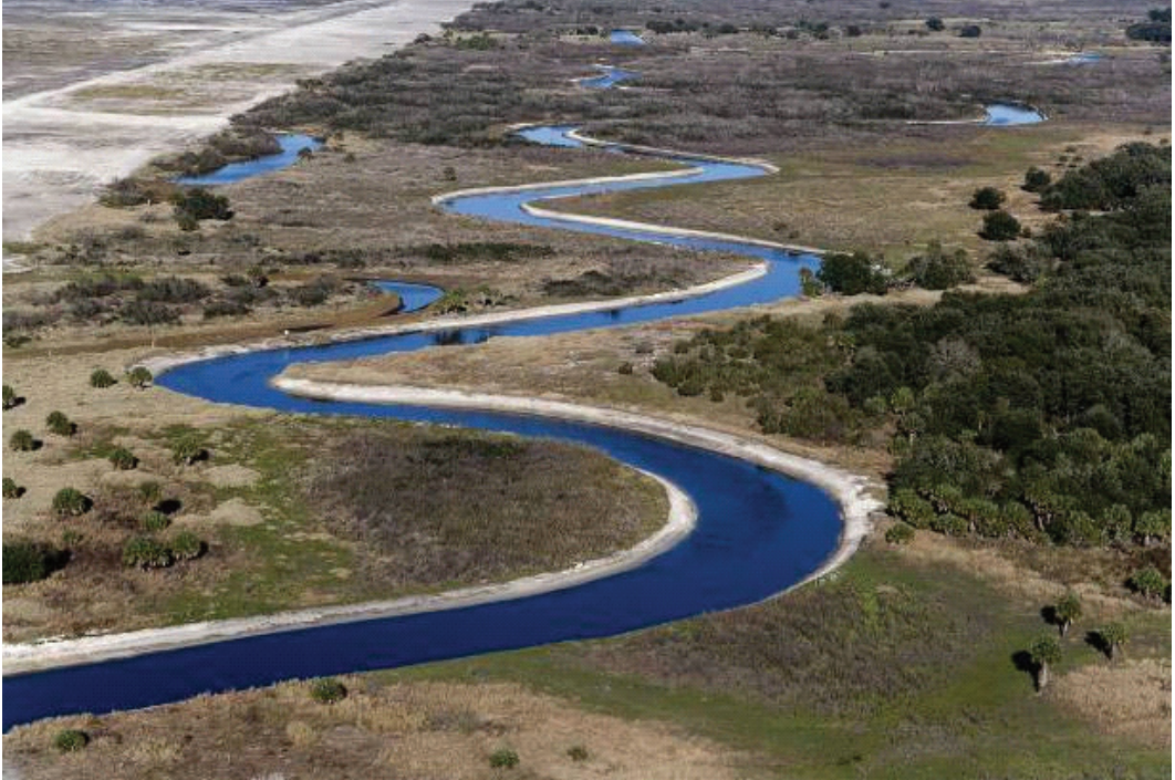
FIGURE 3-15 A restored portion of the Kissimmee River, with the filled C-38 canal in the upper left and the newly re-carved channel of the restored river with an active flood plain on either side.
