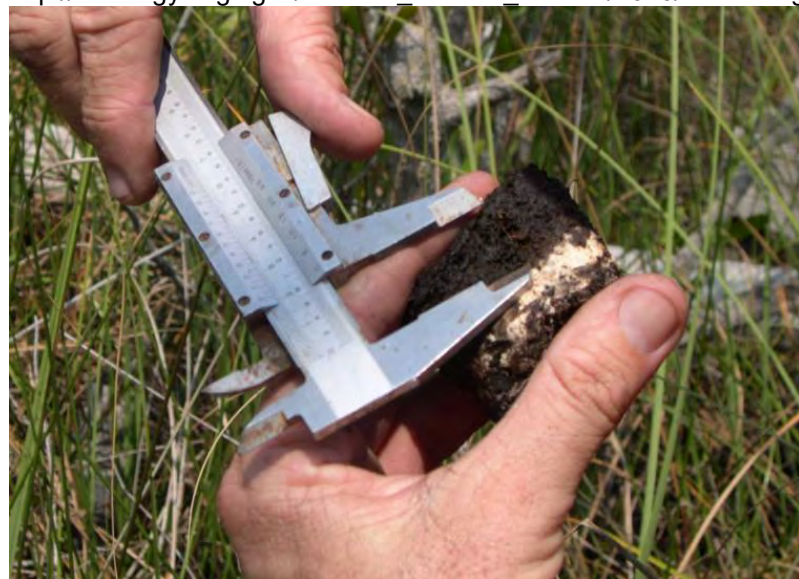
FIGURE 5-9 Measurement of soil accretion using the marker horizon method in Everglades National Park. In this method, researchers place a layer of feldspar clay (visible as a white layer) on the surface of the marsh and later return to measure the soil that has accumulated. The marker horizon method is often used in conjunction with a sediment elevation table (SET) to measure total soil accretion or erosion.
