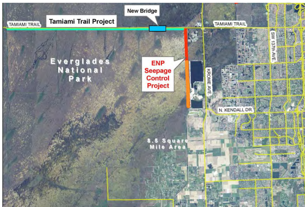
FIGURE 4-20 Position of the 2-mile-long, 35-foot-deep seepage barrier (shown in red), west of the L-31N Canal. The orange line represents a possible 3-mile extension of the project. SOURCE: MacVicar (2014).
