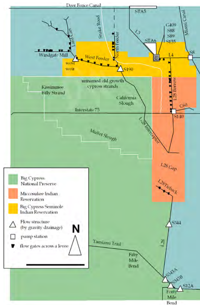
FIGURE 4-28 The Western Glades and the L-28 levee system at the northwest corner of WCA-3A. SOURCE: Florida Gulf Coast University, http://www.fgcu.edu/bcw/Restore/History/History_L28.htm .
