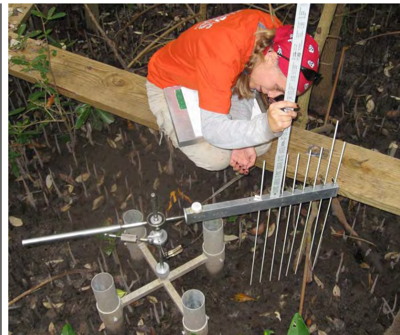
FIGURE 5-8 A sediment elevation table (SET) used to measure changes in the elevation of the soil surface in a mangrove forest in Everglades National Park.
