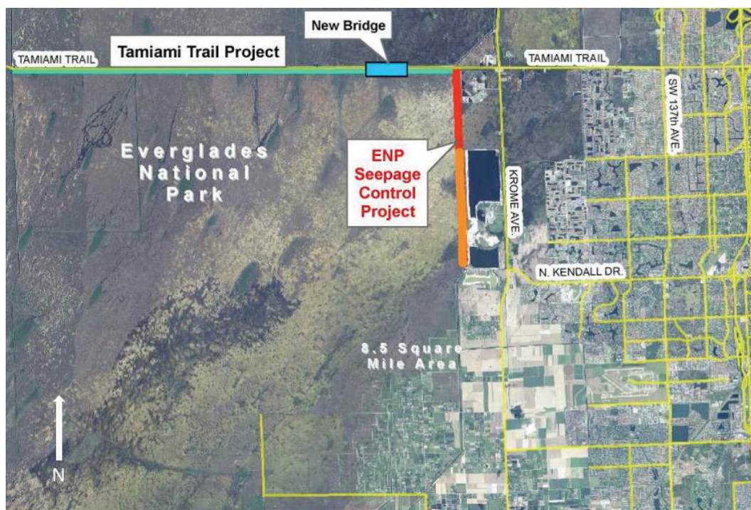
FIGURE 3-26 The 2-mile-long, 35-foot-deep seepage barrier pilot project (shown in red) and the 3-mile extension (shown in orange) are located west of the L-31N Canal. The pilot was completed in 2012, and the 3-mile extension was completed in 2016.
