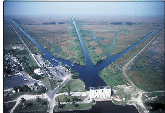
Figure 11. An extensive system of canals, levees, and water control structures has modified Everglades water conditions and provides an inadvertent conduit for pollutant transport. The S9 pump station (foreground) in Broward County discharges stormwater westward from an urban basin into the Everglades (background).
