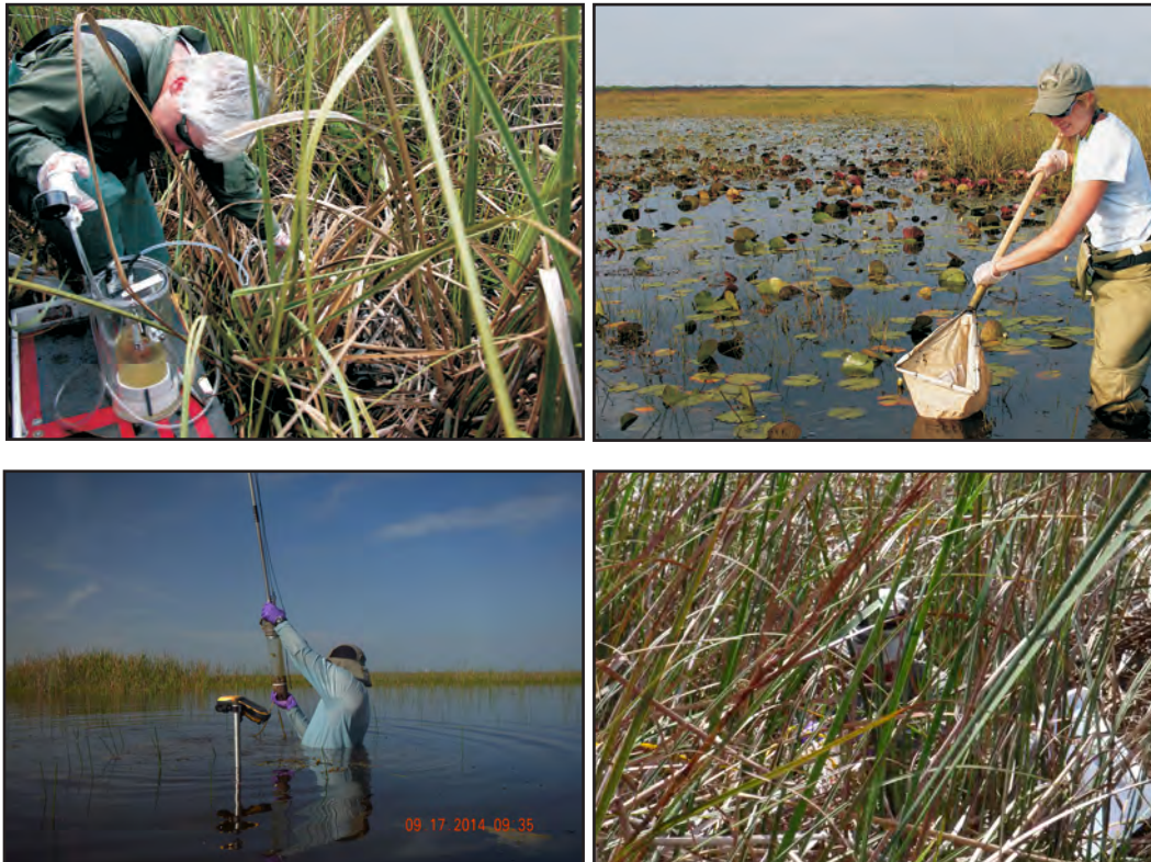
Figure 15. Biogeochemical sampling included surface water (top left), floc and soil (bottom left), and mosquitofish (top right). The surface water sampling apparatus (top left) and soil coring device (bottom left) were designed and constructed for Everglades REMAP. Crews sample in all habitats, including dense sawgrass and cattail mix (bottom right).
