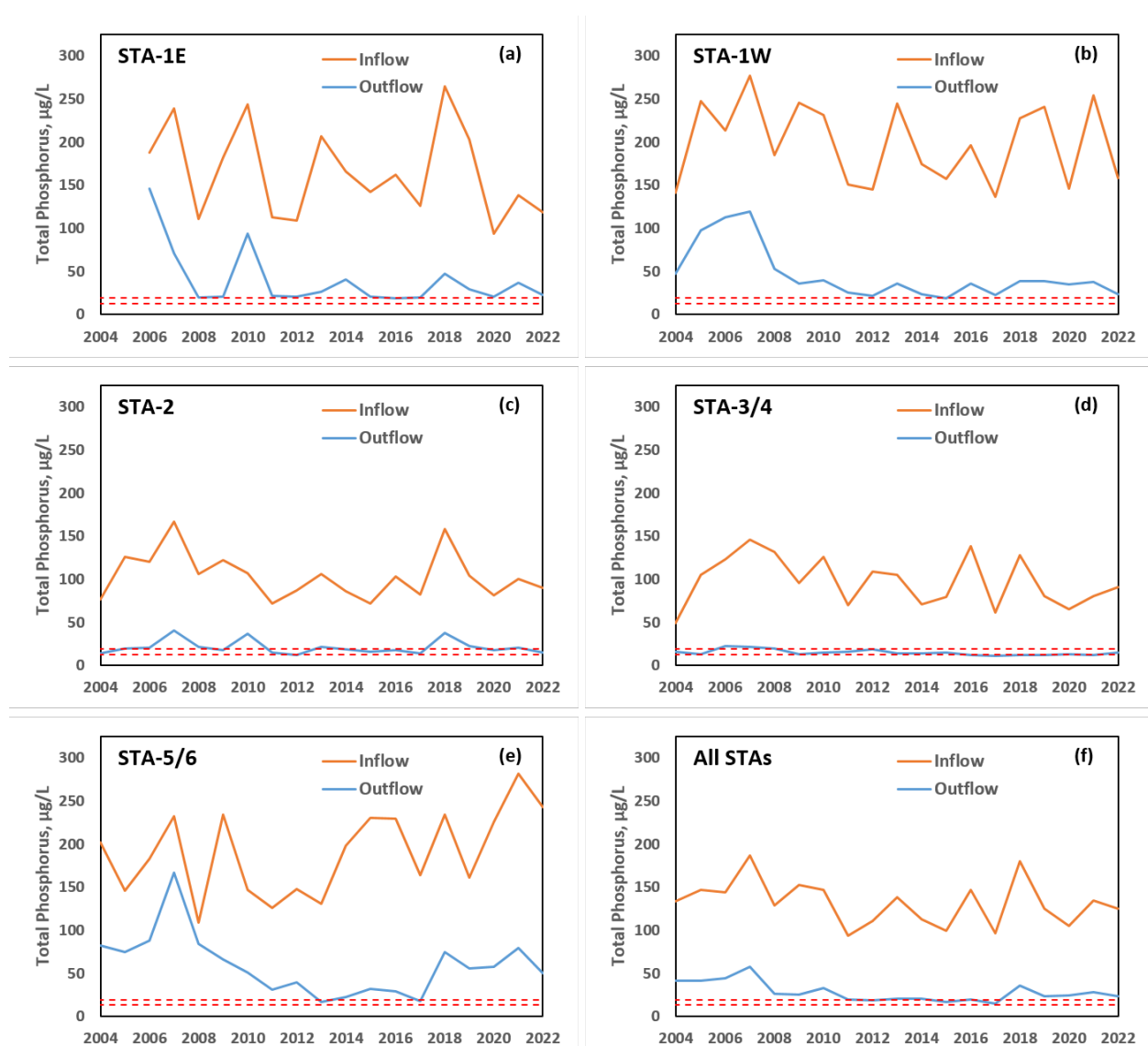
FIGURE B-1 Long-term patterns of annual flow-weighted total phosphorus concentrations on the STA inflow and outflow water during the operation period of WY 2006-2022 for STA-1E and WY 2004-2022 for other STAs. Horizontal dashed line represents the upper and lower limit (19 and 13 µg/L) of total phosphorus concentrations required by WQBEL.
